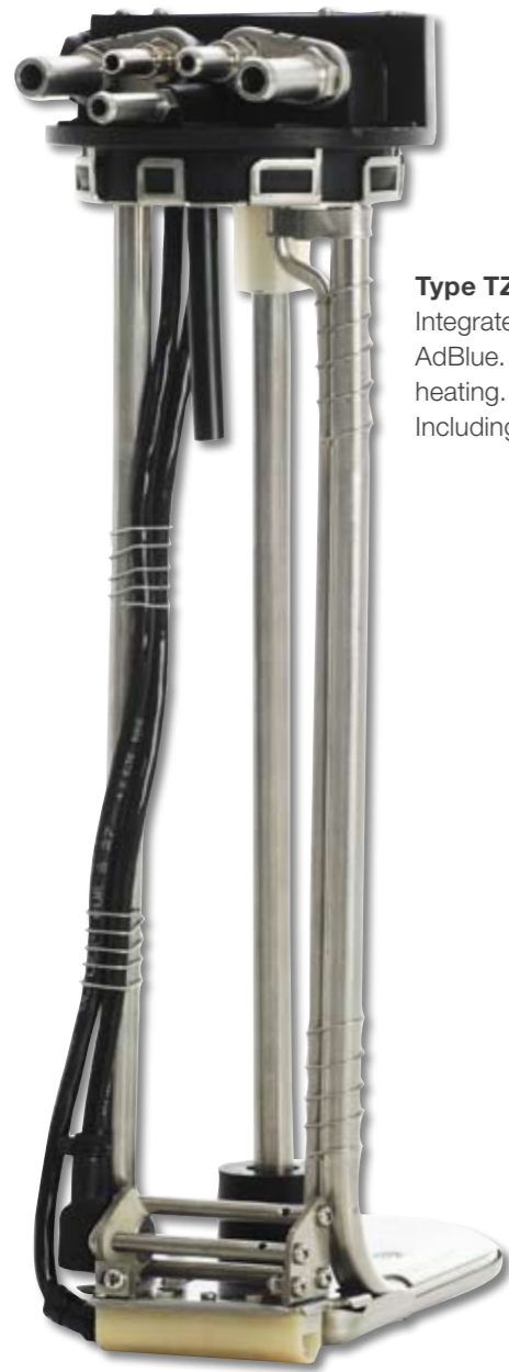
Type TV3S Integrated suction and return of AdBlue. Coolant water circuit for heating. Temperature indication.
